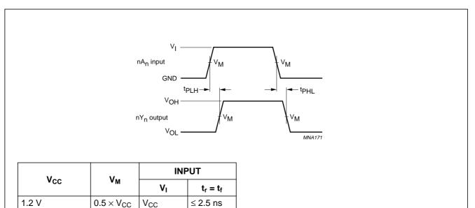
$V_{\text{OL}}$  and  $V_{\text{OH}}$  are typical output voltage drop that occur with the output load.
